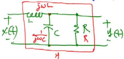
$$\begin{aligned} H(\omega) &= \frac{\frac{1}{j\omega C} \parallel R}{j\omega L + \frac{1}{j\omega C} \parallel R} \\ &= \frac{1}{j\omega L (j\omega C + \frac{1}{R}) + 1} \\ &= \frac{1}{(1 - \omega^2 LC) + j\omega \frac{L}{R}} \\ |H(\omega)| &= \frac{1}{\sqrt{(1 - \omega^2 LC)^2 + (\omega \frac{L}{R})^2}} \end{aligned}$$
